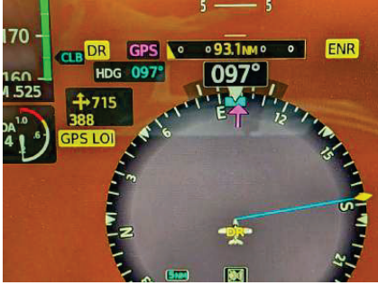
Example of the GPS spoofing that occurred over the Black Sea. Thankfully Amir was prepared and had already calculated expected times and distances (with the wind and speed factored in) to the navigation points.
